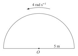
A uniform semicircular lamina has radius 5 m. The lamina rotates in a horizontal plane about a vertical axis through O, the mid-point of its diameter. The angular speed of the lamina is  $4 \, \text{rad s}^{-1}$  (see diagram). Find
