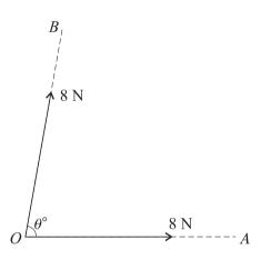
Two forces, each of magnitude 8 N, act at a point in the directions OA and OB. The angle between the forces is  $\theta^{\circ}$  (see diagram). The resultant of the two forces has component 9 N in the direction OA. Find
