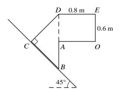
The diagram shows the cross-section *OABCDE* through the center of mass of a uniform prism on a rough inclined plane. The portion *ADEO* is a rectangle in which AD = OE = 0.6 m and DE = AO = 0.8 m; the portion *BCD* is an isosceles triangle in which angle *BCD* is a right angle, and *A* is the mid-point of *BD*. The plane is inclined at 45° to the horizontal, *BC* lies along a line of greatest slope of the plane, and *DE* is horizontal.
