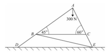
The framework stands, in a vertical plane, on rough horizontal ground. A load of 300 N is hung at A. The framework remains in equilibrium with BC horizontal. By considering the forces acting at A, find the forces in each of the rods AB and AC. (7 marks)
