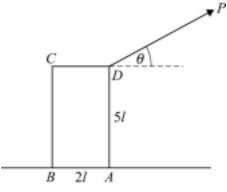
This force acts as shown in the diagram where *ABCD* is a vertical cross section through the centre of mass of the cuboid.
