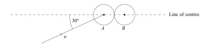
The coefficient of restitution between A and B is e.
