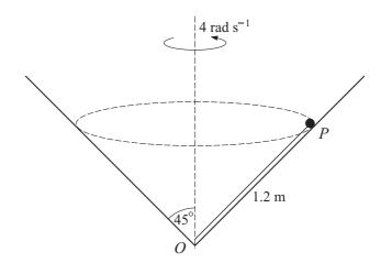
A hollow cone with semi-vertical angle  $45^{\circ}$  is fixed with its axis vertical and its vertex O downwards. A particle P of mass 0.3 kg moves in a horizontal circle on the inner surface of the cone, which is smooth. P is attached to one end of a light inextensible string of length 1.2 m. The other end of the string is attached to the cone at O (see diagram). The string is taut and rotates at a constant angular speed of  $4 \, \text{rad s}^{-1}$ .
