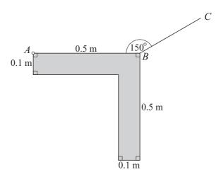
A uniform lamina of weight 9 N has dimensions as shown in the diagram. The lamina is freely hinged to a fixed point at A. A light inextensible string has one end attached to B, and the other end attached to a fixed point C, which is in the same vertical plane as the lamina. The lamina is in equilibrium with AB horizontal and angle  $ABC = 150^{\circ}$ .
