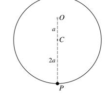
A uniform solid sphere with centre *C*, radius 2*a* and mass 3*M*, is pivoted about a smooth horizontal axis and hangs at rest. The point *O* on the axis is vertically above *C* and OC = a. A particle *P* of mass *M* is attached to the sphere at its lowest point (see diagram). Show that the moment of inertia of the system about the axis through *O* is  $\frac{84}{5}Ma^2$ . [4]
