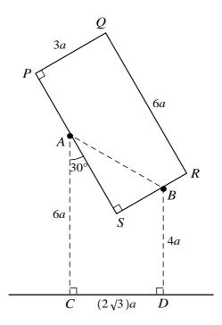
The points C and D are at a distance  $(2\sqrt{3})a$  apart on a horizontal surface. A rough peg A is fixed at a vertical distance 6a above C and a smooth peg B is fixed at a vertical distance 4a above D. A uniform rectangular frame PQRS, with PQ = 3a and QR = 6a, is made of rigid thin wire and has weight W. It rests in equilibrium in a vertical plane with PS on A and SR on B, and with angle  $SAC = 30^{\circ}$  (see diagram).
