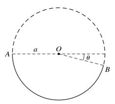
A smooth wire is in the form of an arc AB of a circle, of radius a, that subtends an obtuse angle  $\pi - \theta$  at the centre O of the circle. It is given that  $\sin \theta = \frac{1}{4}$ . The wire is fixed in a vertical plane, with AO horizontal and B below the level of O (see diagram). A small bead of mass m is threaded on the wire and projected vertically downwards from A with speed  $\sqrt{\left(\frac{3}{10}ga\right)}$ .
