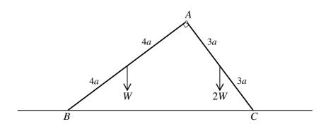
The diagram shows two uniform rods BA and AC, smoothly hinged at A. The rod BA has length 8a and weight W; the rod AC has length 6a and weight 2W. The rods are in equilibrium in a vertical plane with B and C resting on a rough horizontal floor and angle CAB equal to  $90^{\circ}$ . Show that the normal contact force at B is  $\frac{26}{25}W$ . [4]
