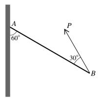
A uniform rod AB of weight W rests in equilibrium with A in contact with a rough vertical wall. The rod is in a vertical plane perpendicular to the wall, and is supported by a force of magnitude P acting at B in this vertical plane. The rod makes an angle of  $60^{\circ}$  with the wall, and the force makes an angle of  $30^{\circ}$  with the rod (see diagram). Find the value of P. [3]
