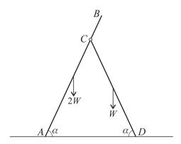
The diagram shows a pair of stepladders modelled by two uniform rods, AB of length 5a and weight 2W and CD of length 4a and weight W, smoothly hinged at C. The stepladders rest on a rough horizontal floor with A fixed so that it cannot slide. The angles CAD and CDA are both equal to  $\alpha$ . By taking moments about A for the system, find the normal contact force at D. [3]
