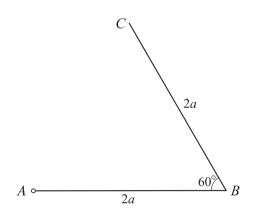
Two uniform rods *AB* and *BC*, each of length 2*a* and mass *m*, are rigidly joined at *B* so that angle  $ABC = 60^{\circ}$  (see diagram). The system is free to rotate in a vertical plane about a horizontal axis though *A*. Show that the moment of inertia of the system about this axis is  $\frac{14}{3}ma^2$ . [3]
