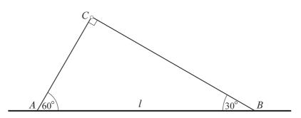
Two straight uniform ladders, *AC* and *BC*, have equal weights *W*. They stand in equilibrium with their feet, *A* and *B*, on rough horizontal ground and their tops freely hinged at *C*. Angle  $CAB = 60^{\circ}$ , angle  $CBA = 30^{\circ}$  and AB = l (see diagram). Find the vertical reactions at *A* and *B*. [6]
