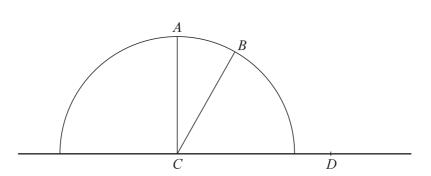
A smooth semicircular cylinder of radius *a* is fixed on a horizontal table with its axis in the plane of the table. *C* is a point on the axis and *CA* is a vertical radius (see diagram). A particle is projected horizontally from *A*, with speed  $\sqrt{(0.4ga)}$ , in a direction perpendicular to the axis. Show that the particle leaves the surface with speed  $\sqrt{(0.8ga)}$  at the point *B* where  $\cos ACB = 0.8$ . [7]
