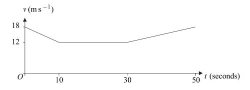
(a) During the first stage of the motion, the coach decelerates at a constant rate of  $a \,\mathrm{m\,s^{-2}}$  for 10 seconds until it reaches a velocity of  $12 \,\mathrm{m\,s^{-1}}$ .
