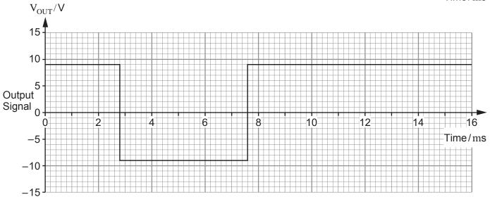
(a) What type of Schmitt trigger would be required to produce this output? [1]
