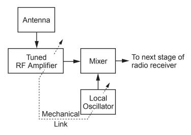
(i) The tuned RF amplifier has been tuned to a frequency of 1.680 MHz. The local oscillator output is measured at 2.145 MHz. What **four** frequency signals will be present at the output of the mixer?
