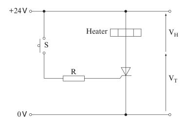
(i) Complete the table by adding the values of  $V_T$  and  $V_H$  when switch  $S_1$  is closed and then re-opened. The thyristor is initially switched **off**. [3]
