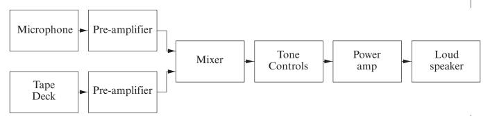
(a) The microphone pre-amplifier is a 2-stage amplifier with an overall gain of 2500.
