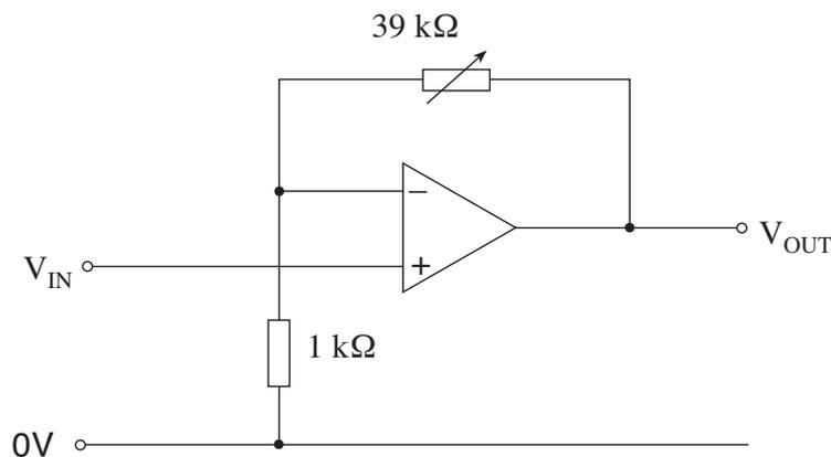
The op-amp is powered from a ±12V supply and saturation occurs at ±11V.
