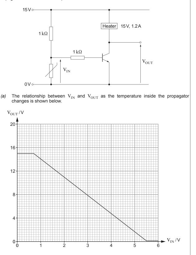
Use the graph to determine the minimum value of  $\ensuremath{V_{\mathrm{IN}}}$  required to saturate the transistor. [1]
