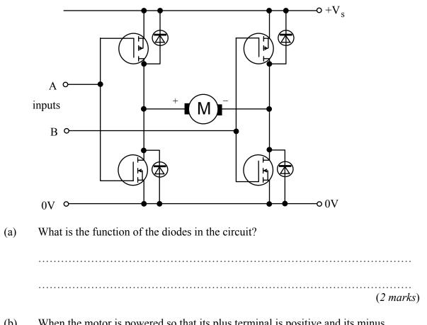
5 (b) When the motor is powered so that its plus terminal is positive and its minus terminal is negative, the motor rotates clockwise. Taking logic 1 as positive and logic 0 as 0V, complete the truth table for the inputs A and B.
