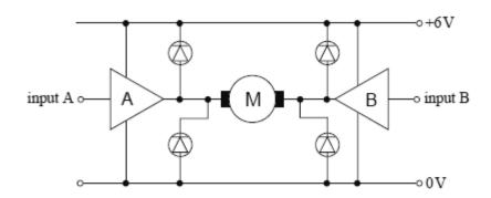
A and B are both high current switching circuits. Each has a truth table as shown below.
