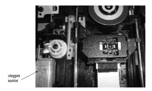
The position of the head is controlled by a stepper motor in the bottom left-hand corner of the photograph. Give two reasons, with supporting explanations, why a conventional motor would not be suitable for controlling the position of the CD-ROM drive head.
