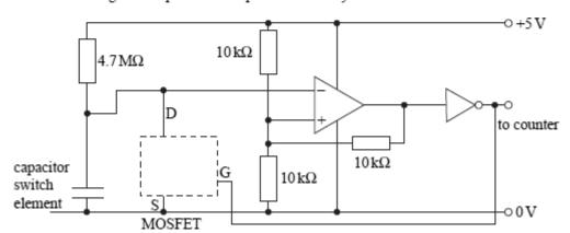
(a) Draw the symbol for the MOSFET in the space provided on the circuit diagram.
