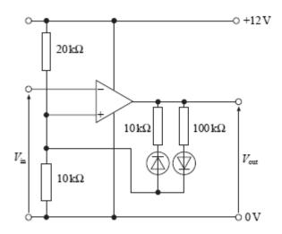
Assume that the op-amp is ideal and the diodes have no forward voltage drop and zero reverse leakage current.
