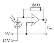
The photodiode current in the dark is  $0.1\,\mu A$  and in the light is  $6\,\mu A$ .
