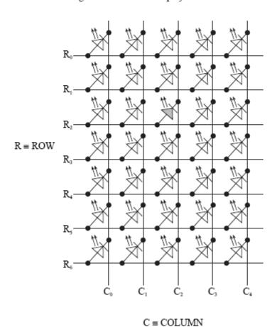
Explain how the LED shaded in the diagram above can be lit.
