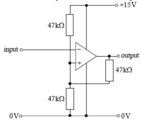
2 (b) (i) Show, by calculation, that if the output is +15V, the input must be less than +10V.
