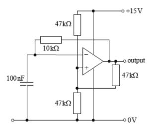
Hence, by comparison with a 555 timer, or otherwise, calculate the time period of the pulses from the output of the circuit.
