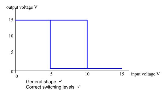
(d) (Capacitor charges and discharges between <sup>1</sup>/<sub>3</sub> and <sup>2</sup>/<sub>3</sub> of supply voltage)
