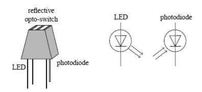
4 (a) The LED has a forward voltage of 1.6V at its maximum working current of 25 mA. The LED is powered from a 5V supply. Using a calculation, select a preferred value for the series resistor.
