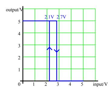
Has two switching levels, ✓ output goes low when upper level is exceeded, ✓ output goes high when input goes below the lower switching level, ✓ diagram completed correctly ✓
