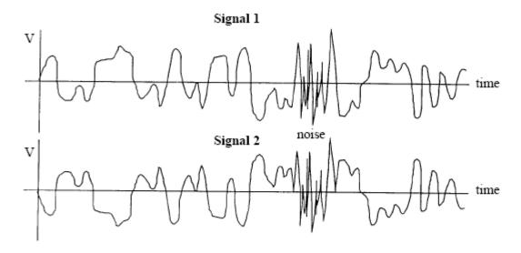
Signal 1 is connected to input A of a summing amplifier. Signal 2 is passed through an amplifier with a voltage gain of -1 and then connected to input B of the summing amplifier, as shown in the diagram below.
