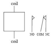
The coil is powered when the monostable output goes high. Which two connections would be used to switch on the lamp?
