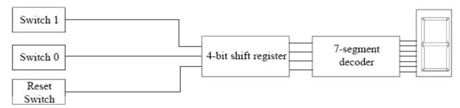
When switch 1 is pressed, the serial input to the shift register is set to logic 1 and a clock pulse is generated to enter the logic 1 into the shift register.
