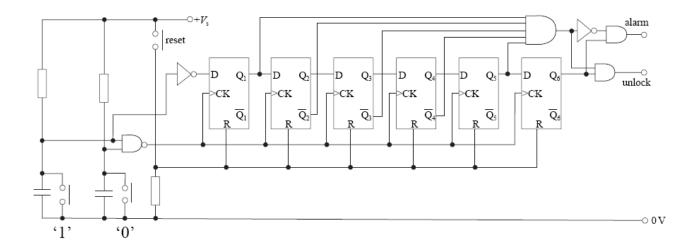
To operate the lock, the circuit is first reset and then a binary number is entered by pressing the '1' and '0' switches. If an incorrect number is entered an alarm is sounded.
