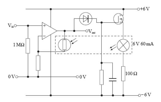
The lamp and LDR are in a sealed container so that only light from the lamp illuminates the LDR.
