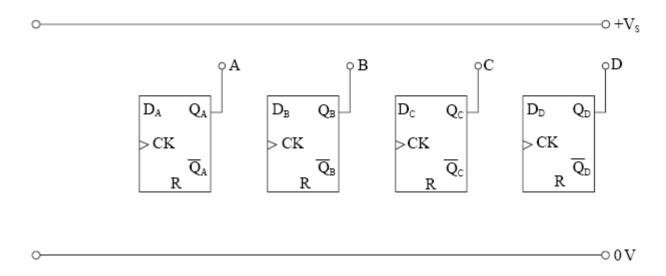
(ii) If the reset terminals of the D-type flip-flops are active high, mark onto the diagram above where you would connect the reset switch and any other components that you need.
