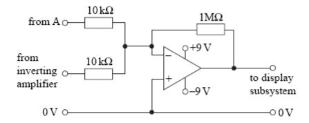
Label the virtual earth point on the amplifier with the letter X.
