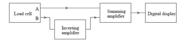
The load cell has a differential output and when there is no force on the load cell, outputs A and B are both at 0 V. When there is a force on the load cell, then output A produces an output of -v and output B produces an output of +v, where v is a small voltage which is proportional to the force on the load cell.
