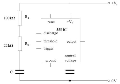
5 (d) (ii) Given the values shown on the circuit diagram for R<sub>A</sub> and R<sub>B</sub>, calculate the value of C required to give an output frequency of 2 Hz.
