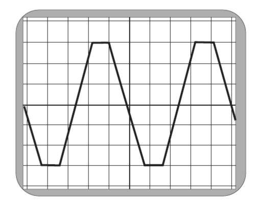
State one electrical property of the amplifier system that causes this distortion.
