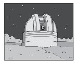
The dome is positioned and opened using large 'mains' powered conventional motors. Stepper motors are used to position the telescope.
