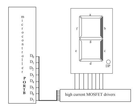
**5 (b)** The outputs from PORTB are connected to the 7-segment display elements via the MOSFET drivers as shown below.
