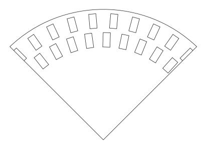
Each circle of slots is read optically using an infra-red LED and photodiode, as shown in the diagram below.
