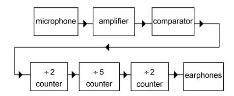
**2 (b) (i)** If the system receives ultrasonic waves at a frequency of 48 kHz, calculate the frequency of the signal at the earphones.
