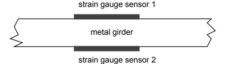
When the girder bends, the resistance of sensor 1 decreases and the resistance of sensor 2 increases.
