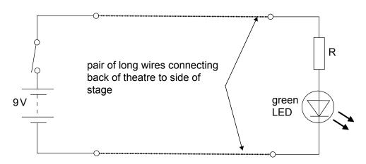
3 (a) Why is it important that the battery is connected the correct way round?
