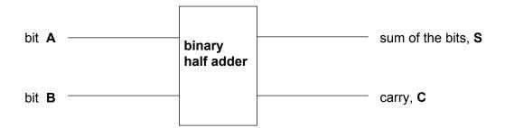
The device operates as shown in the following truth table.
