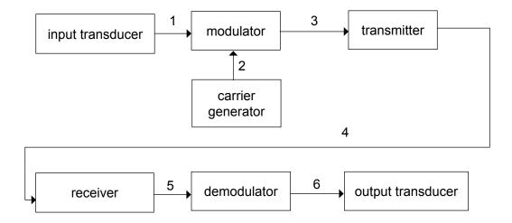
1 (a) The type of signal at number 1 is an information signal and at number 3 it is a modulated carrier wave.State the type of signal that could be at
