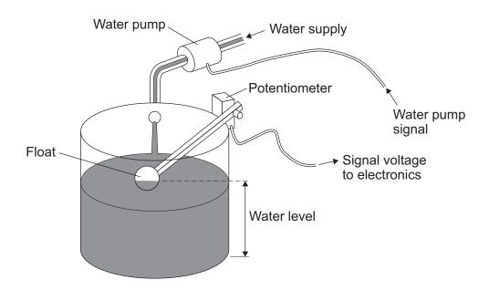
The water level is monitored by a float attached to a potentiometer, so that as the water level rises the voltage from the potentiometer increases.
