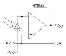
When the photo diode is illuminated the current passing through it is  $10\,\mu\text{A}$  and when it is in the dark the current is zero.
