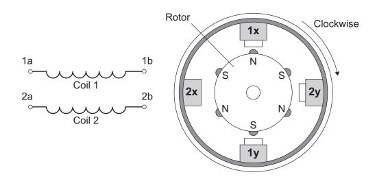
The table below shows the relationship between the current flow through the coils and the magnetic fields created. For example, in the first row, if current passes from terminal a to terminal b in coil 1, then the electromagnet 1x becomes South and electromagnet 1y becomes North.
