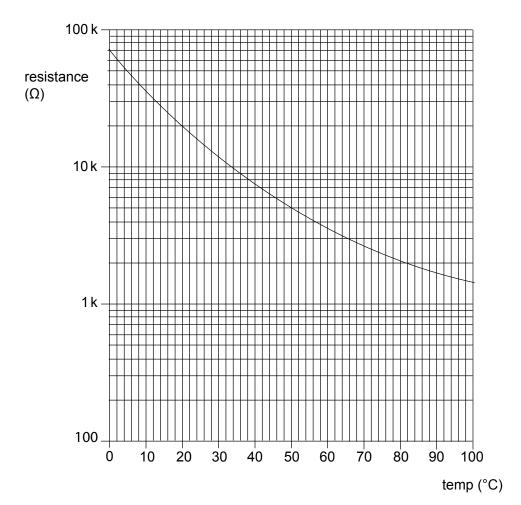
**4 (c)** Calculate the value of R that would make the comparator switch at 20°C.
