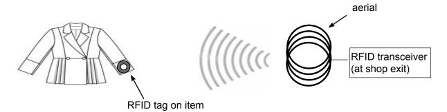
The aerial in the transceiver transmits a signal which activates the tag. The tag then transmits data to the transceiver. The frequency of the signals is typically 13.56 MHz. The transceiver's aerial is made of a coil of wire, which also acts as the inductor for the tuned circuit.
