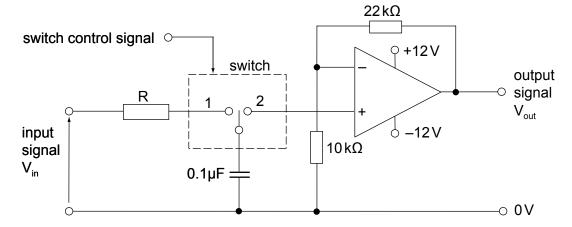
The control signal changes the switch between positions 1 and 2.
