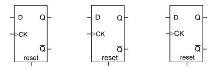
**3** (a) (i) On the diagram of the binary counter above, show how these flip-flops must be connected to form a 3-bit binary up-counter. Label the input from the astable and the three outputs X, Y and Z.
