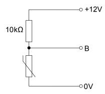
6 (a) The thermistor shown above has a resistance of 45 kΩ at 0 °C, 20 kΩ at 25 °C, and 1 kΩ at 100 °C.
