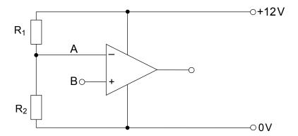
Calculate and choose values of resistors, in the  $1k\Omega$  to  $10k\Omega$  range, for the circuit that will make the comparator switch at  $25\,^{\circ}$ C. Label these on the diagram.
