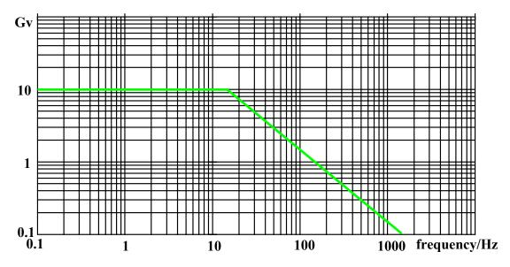
horizontal line to about 10-20Hz ✓ at a gain of 10 ✓ diagonal line - decreasing (at about 10 per decade) ✓
