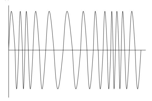
constant amplitude ✓ varying frequency ✓ in phase with info ✓ (3 marks)
