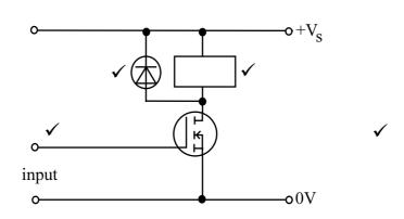
Input to gate and no series resistor, MOSFET symbol correct, relay in drain lead, diode across relay.
