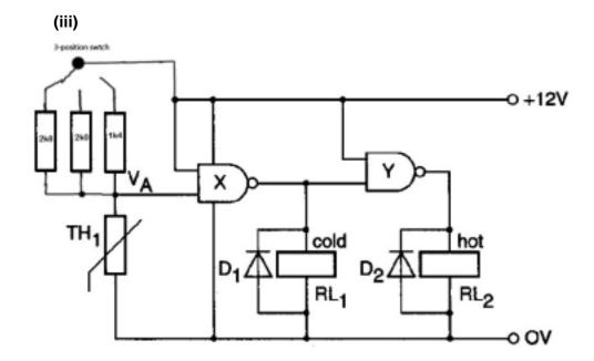
As above or similar. (1) for each correct resistor value, where  $2k8 = 35^{\circ}$   $2k0 = 40^{\circ}$   $1k4 = 45^{\circ}$
