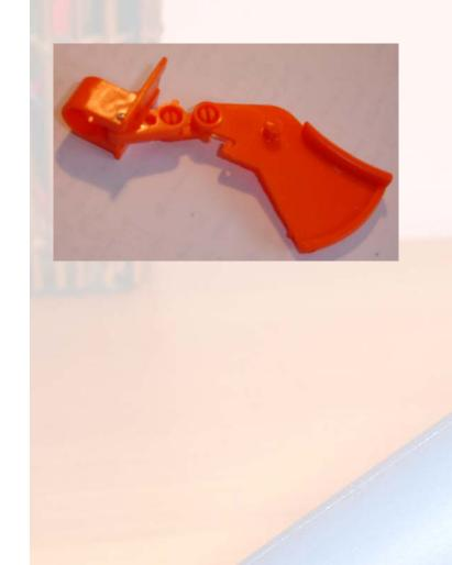
The material used in the trigger mechanism is Acrylonitrile Butadiene Styrene comonomer (ABS), which is appropriate to the requirements of the trigger mechanism; properties include:
