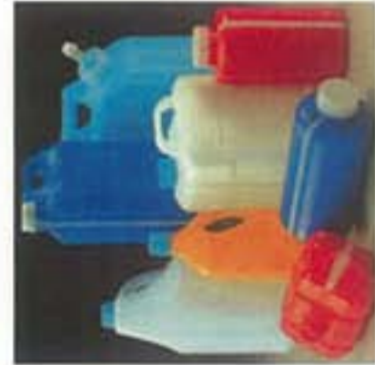
Fig 3: A selection of products manufactured using Blow moulding techniques.
