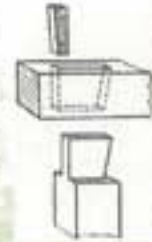
Dovetailed and wedged tenon
