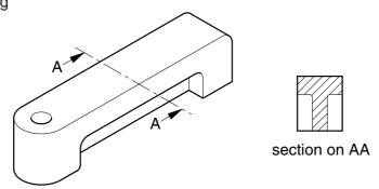
Runner for sliding doors Process: extrusion
