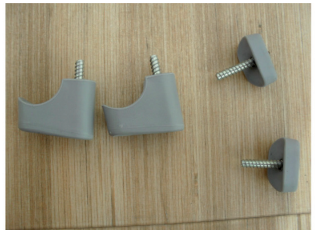
Figure 5 Clamps used to attach frame to seat pad
