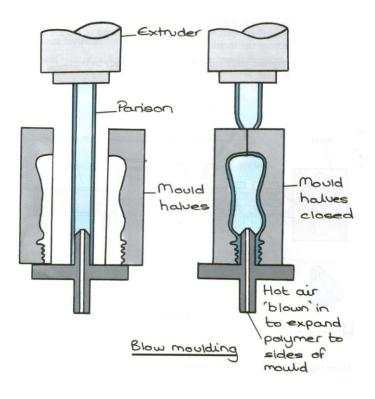
LDPE granules are heated and made into a molten state. The polymer is extruded in a tube form known as a 'Parison'. The mould halves close on the 'Parison' and trap the base together. Air is blown into the Parison which is forced out to the sides of the mould where it cools.The moulds open, releasing the product. Flash is removed.
