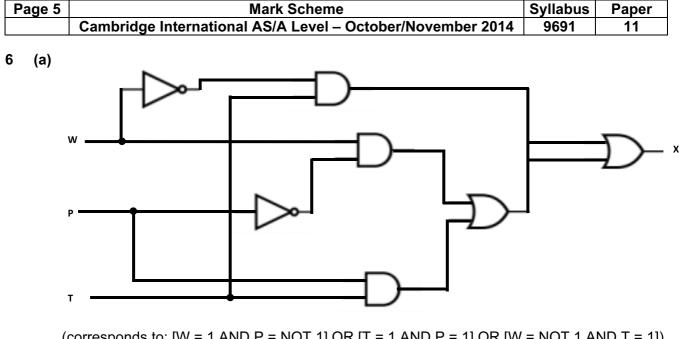
(corresponds to: [W = 1 AND P = NOT 1] OR [T = 1 AND P = 1] OR [W = NOT 1 AND T = 1]) 1 mark for each correct logic gate in correct position – [7]
