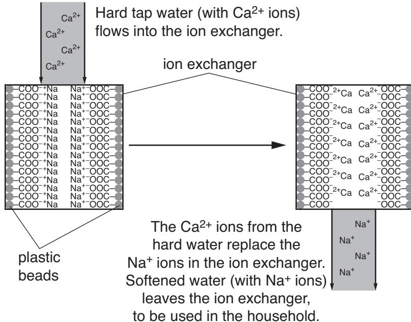
When hard tap water passes through the ion exchanger, the calcium ions from the tap water replace the sodium ions in the ion exchanger. Each calcium ion displaces two sodium ions during this process. the softened water, containing sodium ions in place of calcium ions, can be collected for household use.
