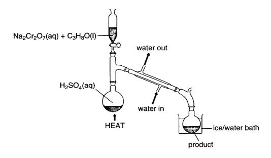
Make up a solution containing 39.3 g of sodium dichromate(VI),  $Na_2Cr_2O_7$ , in 15 cm<sup>3</sup> of water, add 18.0 g of the alcohol,  $C_3H_8O$ , and pour this mixture into the dropping funnel.
