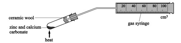
A mixture containing 0.27 g of powdered zinc and 0.38 g of powdered CaCO<sub>3</sub> was heated strongly for two minutes. The volume of gas collected in the 100 cm<sup>3</sup> syringe was then measured. The experiment was then repeated.
