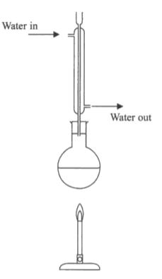
The apparatus has been incorrectly set up in TWO ways. State and explain these mistakes and how they should be corrected. You may assume that the apparatus is suitably clamped and that the reaction mixture contains anti-bumping granules.
