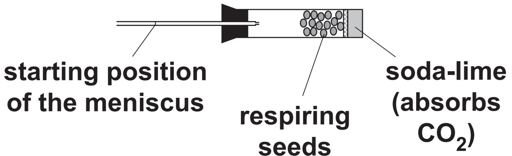
**A student set up the respirometer to measure oxygen consumption.**
