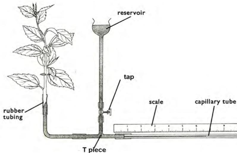
1. Attach the rubber tubing, the capillary tube and the water reservoir to the T piece.
