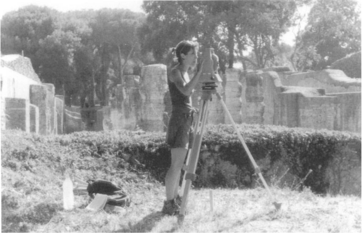
Figure 1 Archaeologist using a Total Station Theodolite to survey and record the site and the surrounding landscape
