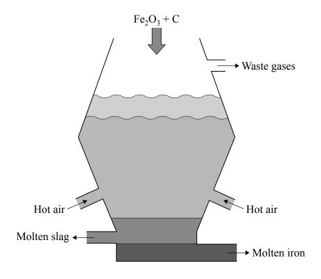
4 (a) A blast furnace is operated as a continuous process.
