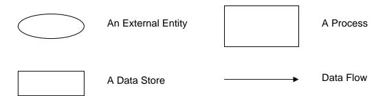
A context diagram (Level 0) is a DFD which shows the entire system as a single process, with data flowing between it and the outside world represented by external entities. The main purpose of a Level 0 DFD is to help fix the boundaries of the system and to show its interaction with external entities.
