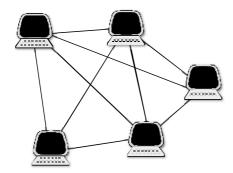
Diagram shows fully connected mesh, a partly connected mesh is acceptable.
