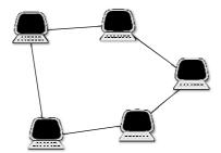
data usually moves in one direction around the ring data sent from one PC will go to all PCs between sender and reciever cable break may not stop the network but speed will drop significantly PCs can be attached via spurs
